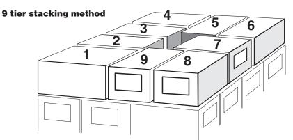
Products that are 8.5' x 11' or can be folded to those dimensions are considered standard IRS products and should be stacked using this 9 tier method.
