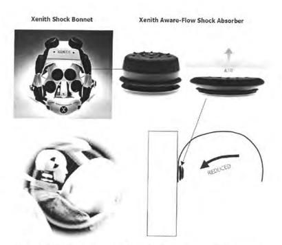
The Xenith Shock Bonnet is a suspension of Aware-Flow Shock Absorbers, which function like automotive air bags. Aware-Flow Shock Absorbers collapse over a prolonged period of time, which minimizes the sudden movement of the head during impact. Aware-Flow Shock Absorbers adapt to impact in order to function over a wide energy range; they refill instantaneously, function over a wide temperature range, and show outstanding multi-impact durability.
