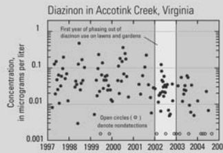
Figure 8-7. From 1997 to 2001, the levels and ranges of diazinon concentrations in Accotink Creek (Potomac River Basin) were relatively similar from year to year, but from 2002 to 2004, diazinon concentrations generally decreased. These decreases correspond to the national reduction in total sales and use of diazinon through this period, although no specific use data were available for the Accotink Creek watershed.
