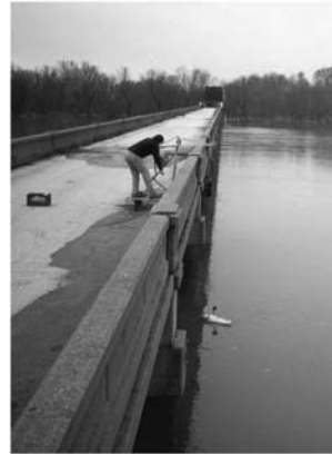
Large streams and rivers required sampling from bridges, boats, or cableways.
