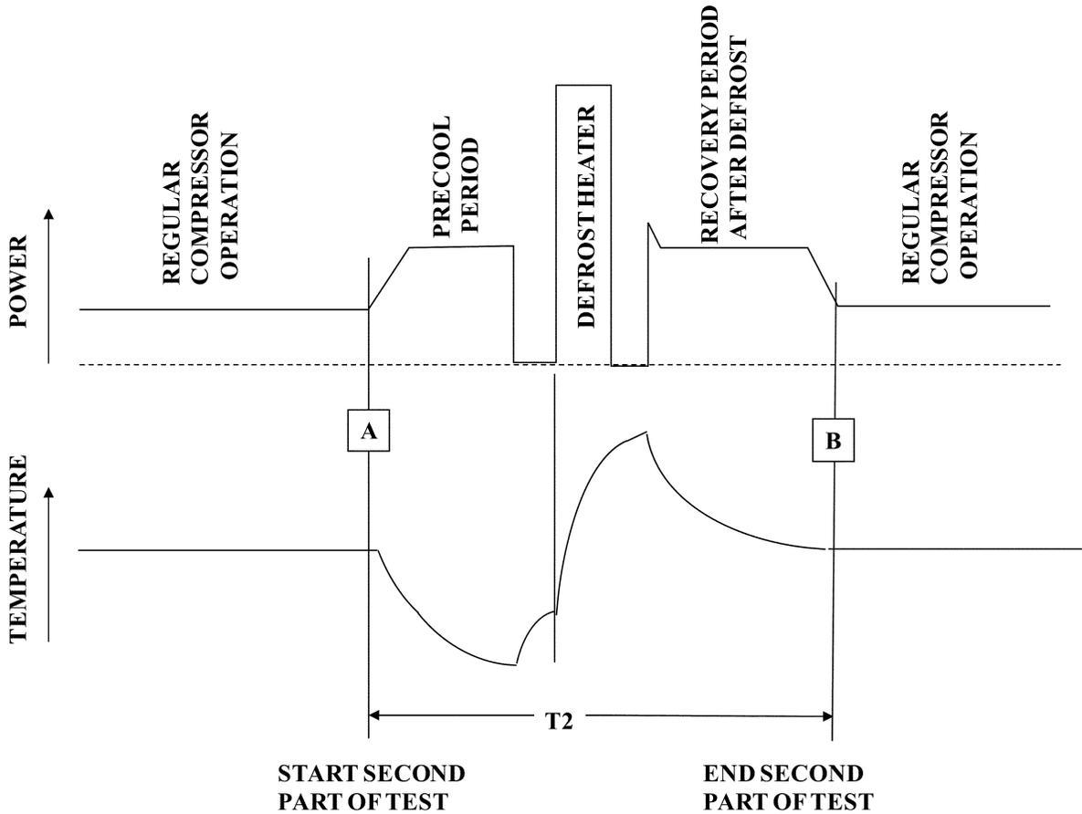
\*Average compartment temperature(s) at times A & B must be within 0.5 °F of the average temperature(s) for the first part of the test.
