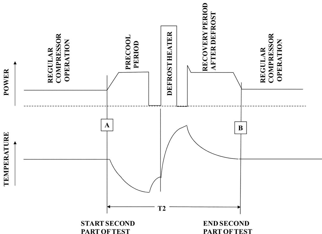
\*Average compartment temperature at times A & B must be within 0.5 °F of the average temperature for the first part of the test.
