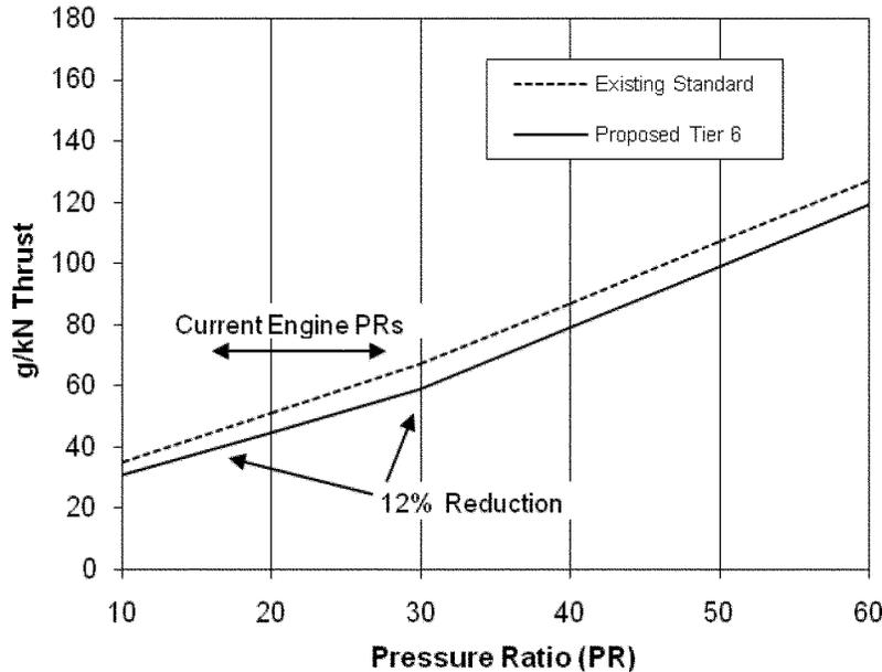
At other thrust ratings the percent reduction between the new Tier 6 and existing EPA NO<sub>x</sub> standards at any pressure ratio becomes progressively smaller as thrust decreases. This is illustrated in Figure 3 for a pressure ratio of 30. This pressure ratio was chosen for the example because, as before, the relative stringency of CAEP NO<sub>x</sub> standards is generally compared at
