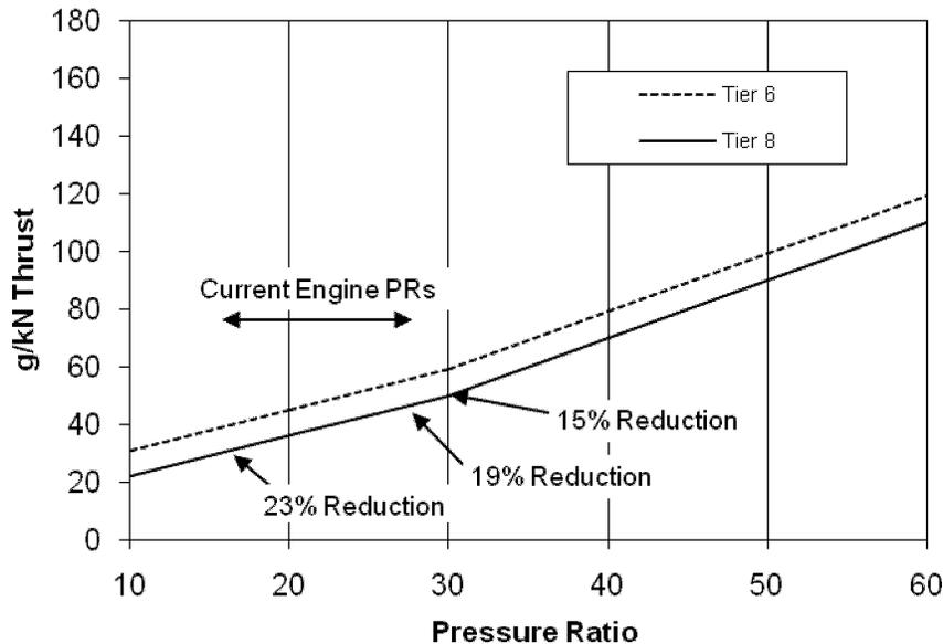
Third, at other thrust ratings the percent reduction between the new Tier 6 and Tier 8 standards at any pressure ratio becomes progressively smaller as thrust decreases. This is illustrated in Figure 6 for a pressure ratio of 30, following the convention described above. Also as shown in the figure for current engines, the reduction ranges
