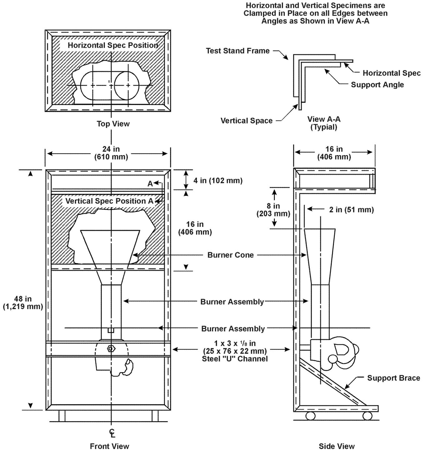
Figure 2: Calorimeter Bracket
