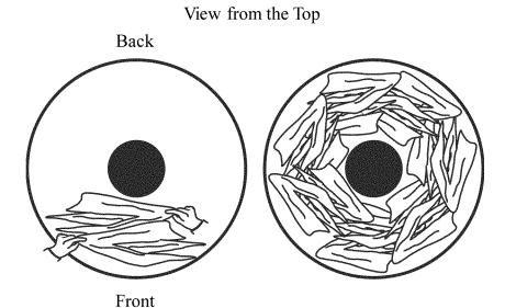
Figure 2.8.3.3—Loading Energy Test Cloths into a Front-Loading Clothes Washer
