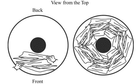
Figure 2.9.2.3—Loading Energy Test Cloths into a Front-Loading Clothes Washer
