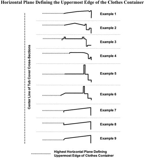
For a front-loading horizontal-axis clothes washer, fill the clothes container to the highest point of contact between the door and the door gasket. If any portion of the door or gasket would occupy the measured volume space when the door is closed, exclude the volume that the door or gasket
