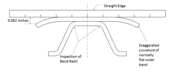
Figure 1 to paragraphs (k)(1)(iii) and (v) of this AD: Cross section of v-band
