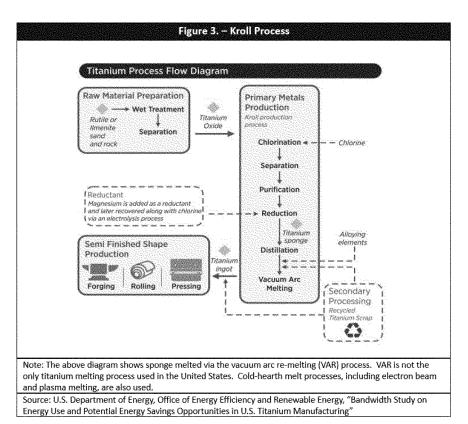
The Kroll process involves several steps. First, a pressurized steel vessel is filled with argon and magnesium enabling the reduction of TiCl<sub>4</sub>.<sup>31</sup> The
