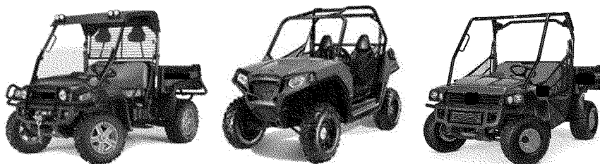
Figure 1. Left to Right: Typical Utility-Type ROV, Typical Recreational-Type ROV, and Typical UTV
