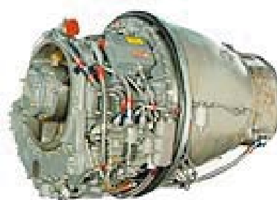
The Teledyne-Ryan J69, jet engine, which the PRC copied in the 1960s.
