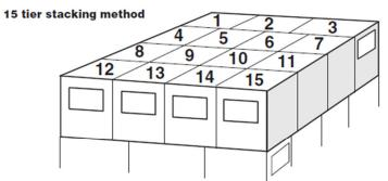
Shipments requiring palletization of cartons for non-Standard (i.e products that are not and can not be folded down to an 8.5' x 11' size without destroying the functionality or integrity of the product) IRS products should be stacked using this 15 tier method.
