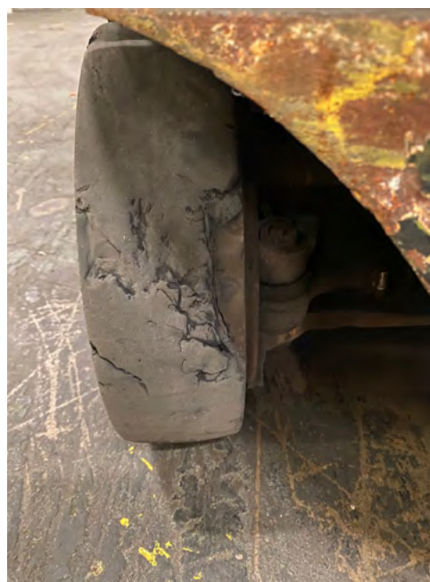
Figure 6. A portion of Tire Missing from A Powered Industrial Truck
