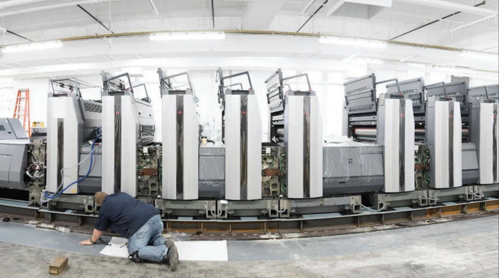
The new 8-color press being installed.
