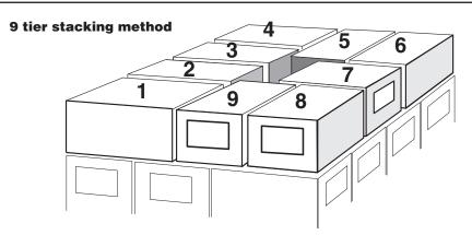
Products that are 8.5' x 11' or can be folded to those dimensions are considered standard IRS products and should be stacked using this 9 tier method.
