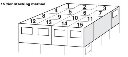
Shipments requiring palletization of cartons for non-Standard (i.e products that are not and can not be folded down to an  $8.5' \times 11'$  size without destroying the functionality or integrity of the product) IRS products should be stacked using this 15 tier method.
