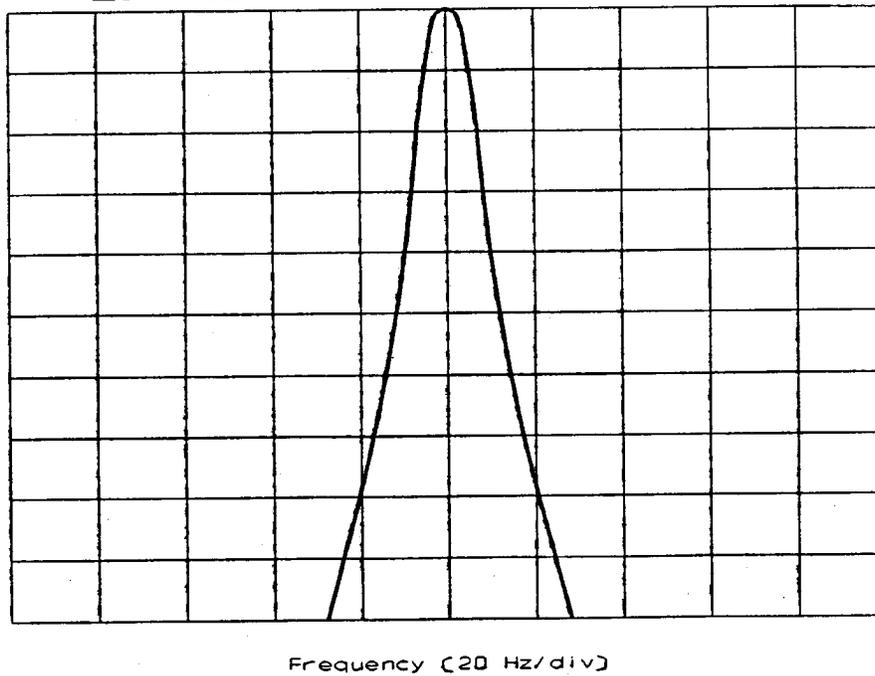
**Figure 4 - Example of EPIRB Carrier Component**
