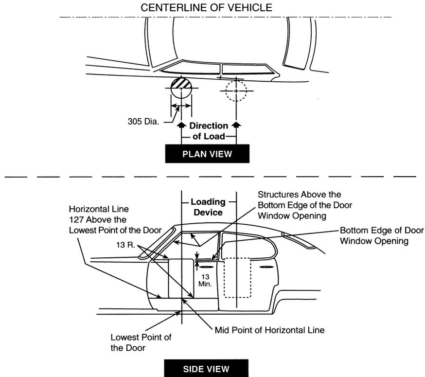
**Figure 1—LOADING DEVICE LOCATION AND APPLICATION TO THE DOOR**
