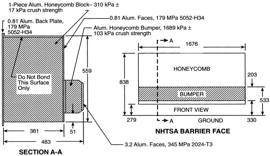
**Figure 2—NHTSA SIDE IMPACTOR – MOVING DEFORMABLE BARRIER**
