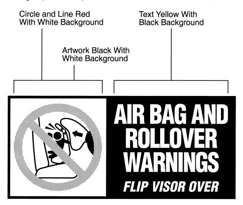
Figure 2. Sun Visor Label Visible When Visor is in Up Position.
