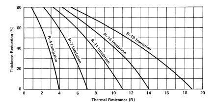
When insulation is installed over the framing members the thermal performance of the insulation is reduced due to compression at the framing members. The Resistance value of the insulation between the framing members is reduced by 12.5 percent for framing members 16" O.C., 8.5 percent for framing members 24" O.C., and 4 percent for framing members 48" O.C.
