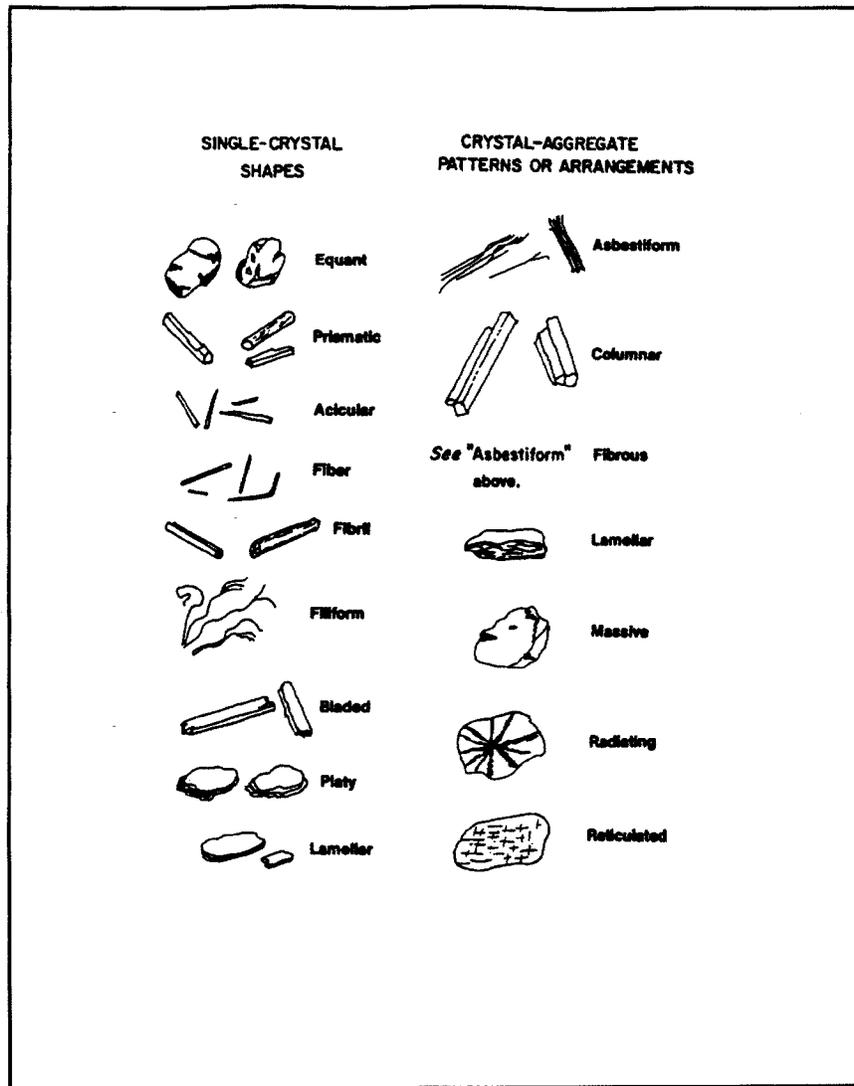
Figure 1. Particle definitions showing mineral growth habits.
