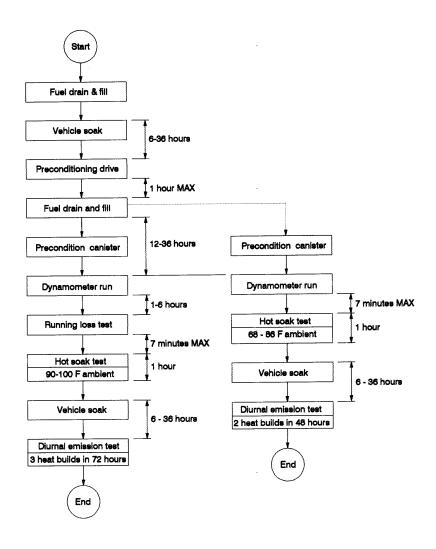
Figure M96-1 Test sequence
