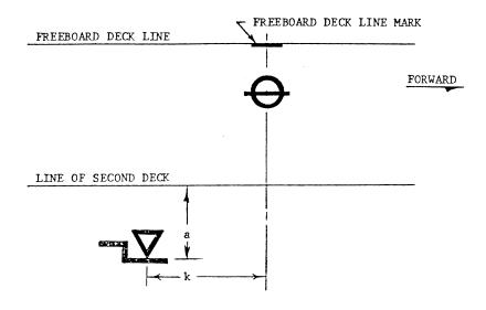
k=a distance between 21 inches and six feet six inches. a=distance derived from Table 69.177(a)(5). (c)—Tonnage mark location if the load line mark is placed as though the second deck were the freeboard deck.
