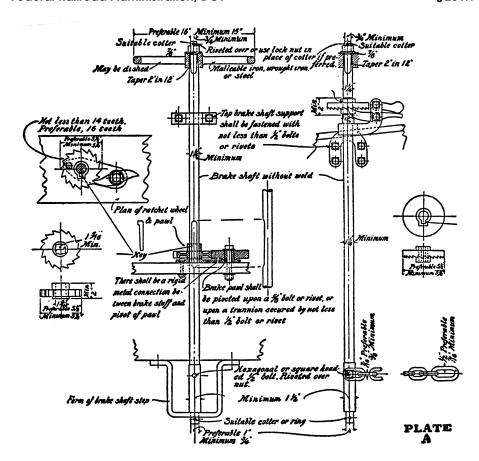
(iv) A brake-shaft step shall support the lower end of brake shaft. A brakeshaft step which will permit the brake chain to drop under the brake shaft shall not be used. U-shaped form of brakeshaft step is preferred. (See plate A.)
