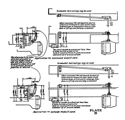
(v) Ends of handles shall extend not less than 4 inches below bottom of end sill or shall be so constructed as to give
