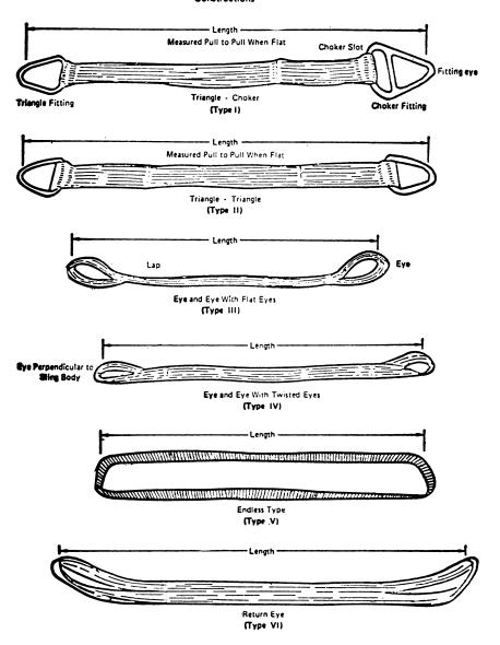
(7) Safe operating temperatures. Synthetic web slings of polyester and nylon shall not be used at temperatures in excess of 180 °F. Polypropylene
