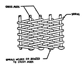
FIG. N-184-2 Metal Mesh Construction
