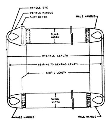
FIG. N-184-1 Metal Mesh Sling (Typical)
