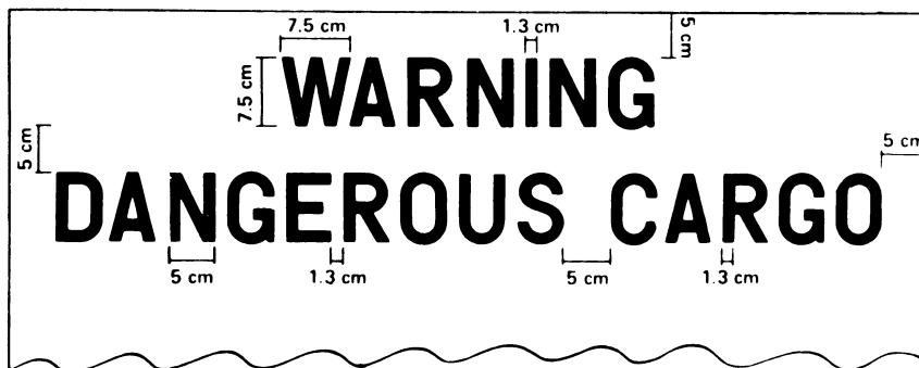
Figure 1 - Minimum Dimensions for Warning Sign
