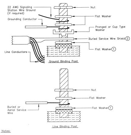
(1) If shoulder is inadequate to support shield or wire add a flat washer.
