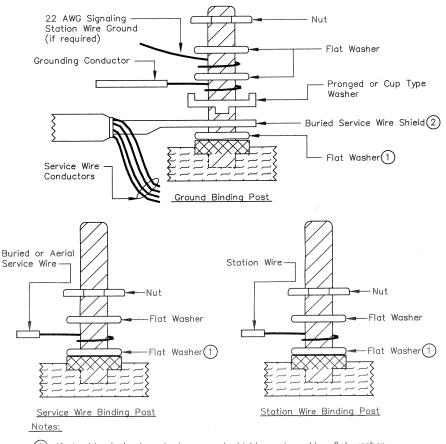
(1) If shoulder is inadequate to support shield or wire add a flat washer.
