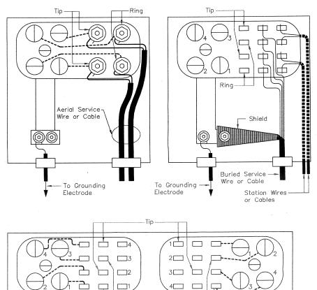
Note: #18 AWG copper-covered steel reinforced aerial service conductors shall not be connected to quick connect terminals. Nonmetallic reinforced aerial service conductors (#22 AWG copper) may be connected to quick connect terminals.
