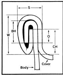
(b) Seamscope or seam projector. Required measurements of the seam include thickness, body hook, and overlap. Seam thickness shall be obtained by micrometer. For cylindrical containers, at least two locations, excluding the side seam juncture, shall be used to obtain the required measurements.
