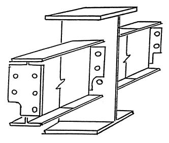
Clipped end connections are connection material on the end of a structural member which has a notch at the bottom and/or top to allow the bolt(s) of the first member placed on the opposite side of the central member to remain in place. The notch(es) fits around the nut or bolt head of the opposing member to allow the second member to be bolted up without removing the bolt(s) holding the first member.
