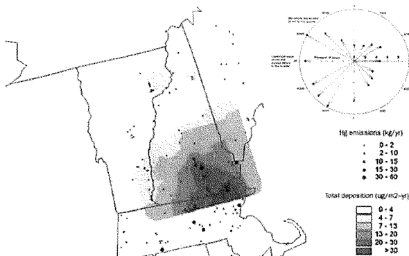
Figure 5. Left, map showing total mercury (Hg) deposition for 2002, estimated using the industrial source complex short-term model, or ISCST3; right, wind rose showing the direction of air flow for May through August 1999 to 2002 in southern New Hampshire, based on weekly wind roses from the NOAA (National Oceanic and Atmospheric Administration) Air Resources Laboratory's READY (Real-time Environmental Applications and Display System) analyses (NOAA 2006).
