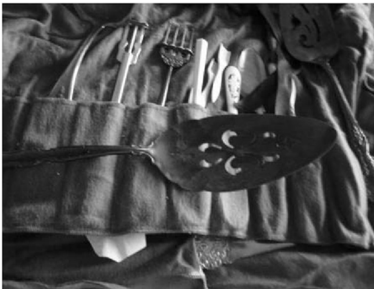
Photo 12—View of a silver plated serving spool that has signs of blackening and pitting marks
