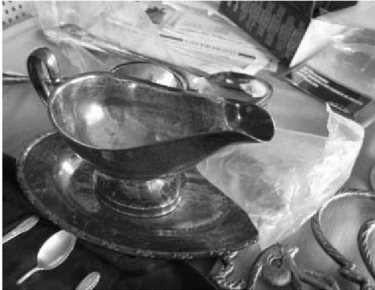
Photo 12—View of a silver plated serving spool that has signs of blackening and pitting marks
