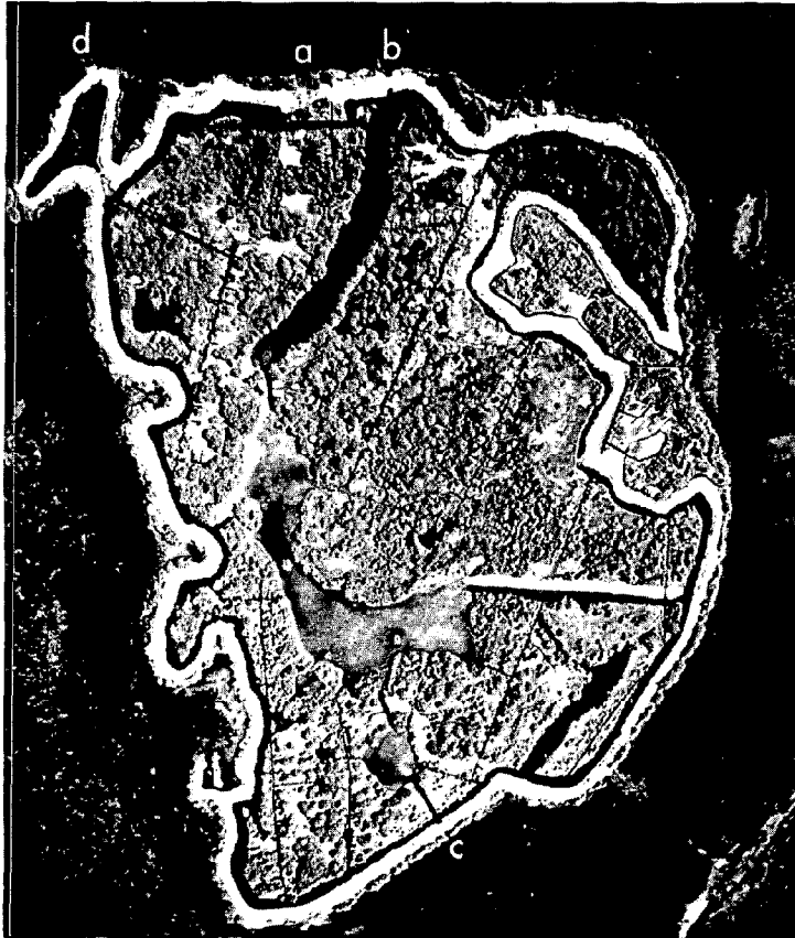
Figure 10. Seasonal impoundment on Gumbo Island, Fla. Water management devices: (a) spillway, the low, grassed-over section of dike; (b) culverts with flash boards; (c) culverts with flap-gate; (d) electric pump, served by underwater cable. (Photo courtesy National Aeronautics and Space Administration.)
