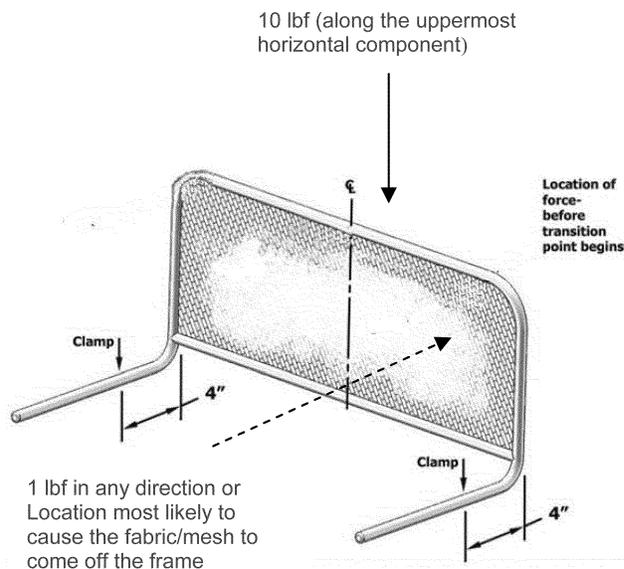
Figure 8: Determining misassembly/functional bed rail test setup
