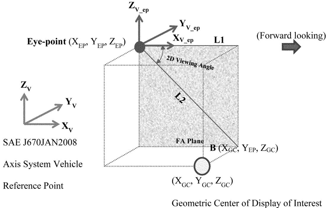
Figure 1. Plane FA Showing Lines 1 and 2 and the 2D Downward Viewing Angle
