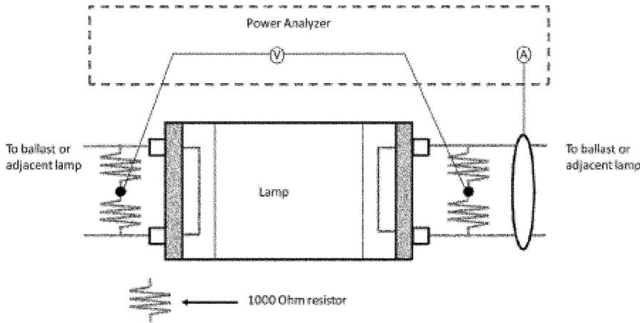
Figure 1: Programmed- and Rapid-Start Ballast Instrumentation Setup
