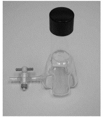
Figure 1. A Baffled Trypsinizing Flask
