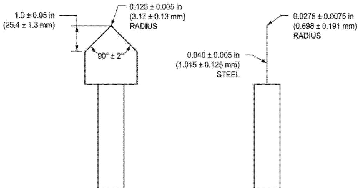
**Figure 8 to Subpart A of Part 1211—Example Test Apparatus for Measurements At
