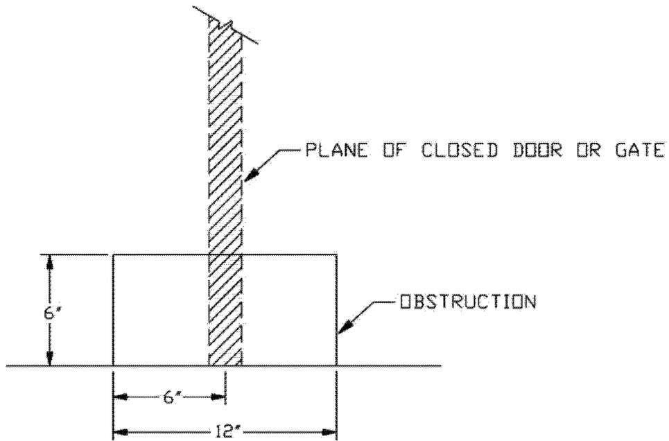
**Figure 4 to Subpart A of Part 1211—Moving Obstruction**
