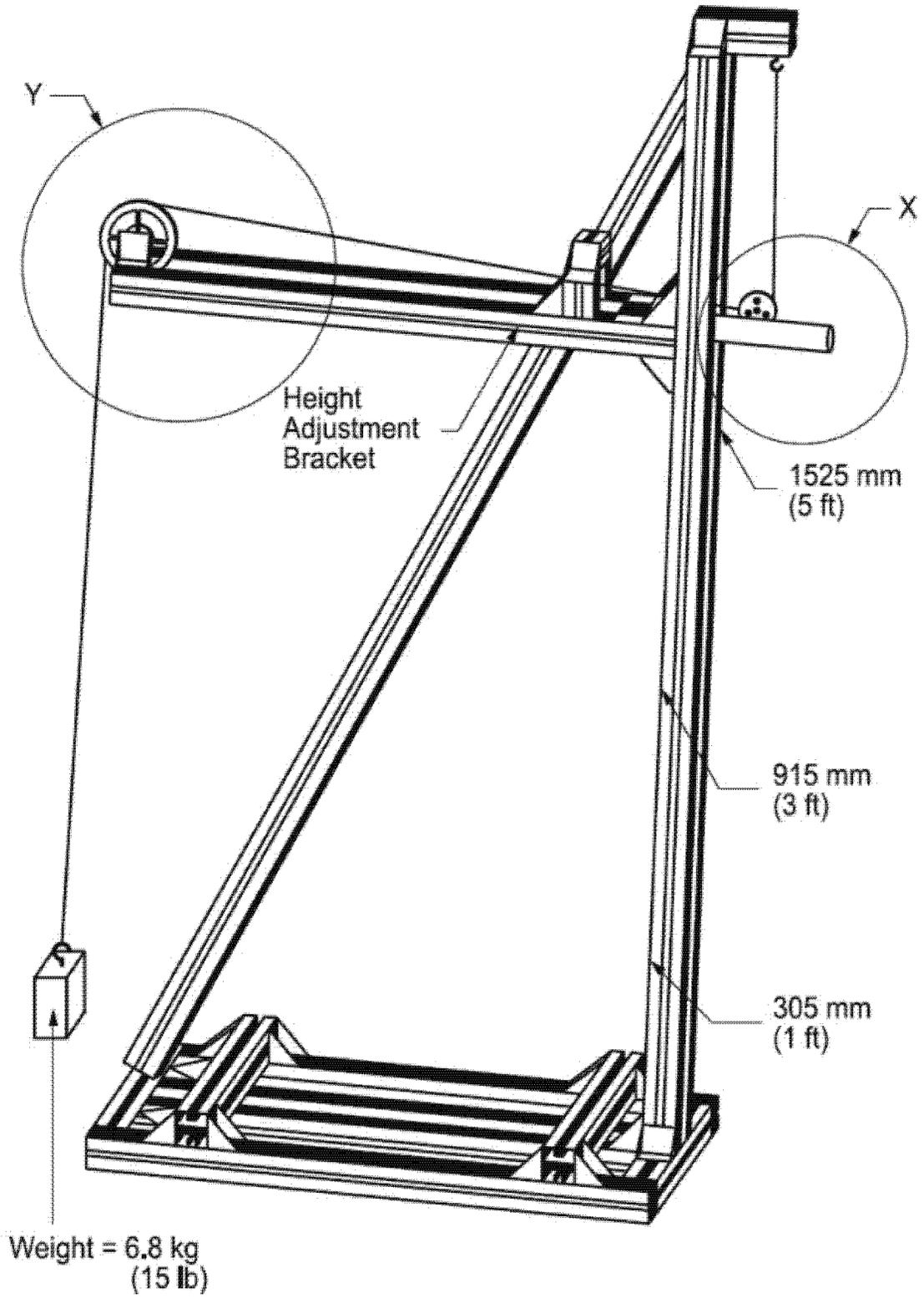
**Figure 10 to Subpart A of Part 1211—Example Test Apparatus for Measurements****At 12 Inches or Greater**
