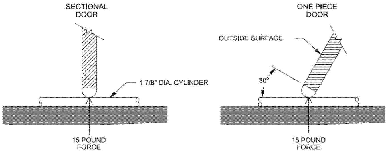
**Figure 7 to Subpart A of Part 1211—PUNCTURE PROBE**
