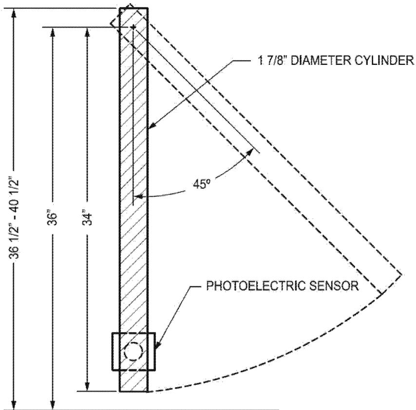
**Figure 5 to Subpart A of Part 1211—Ambient Light Test**
