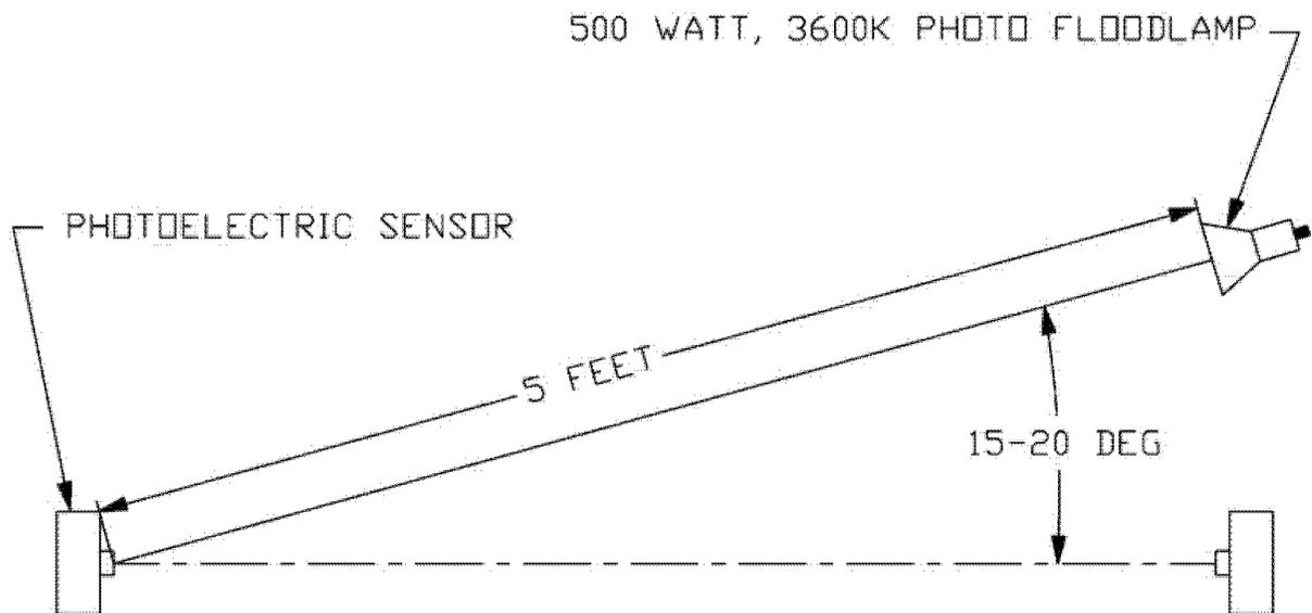
**Figure 6 to Subpart A of Part 1211—Edge Sensor Normal Operation Test**
