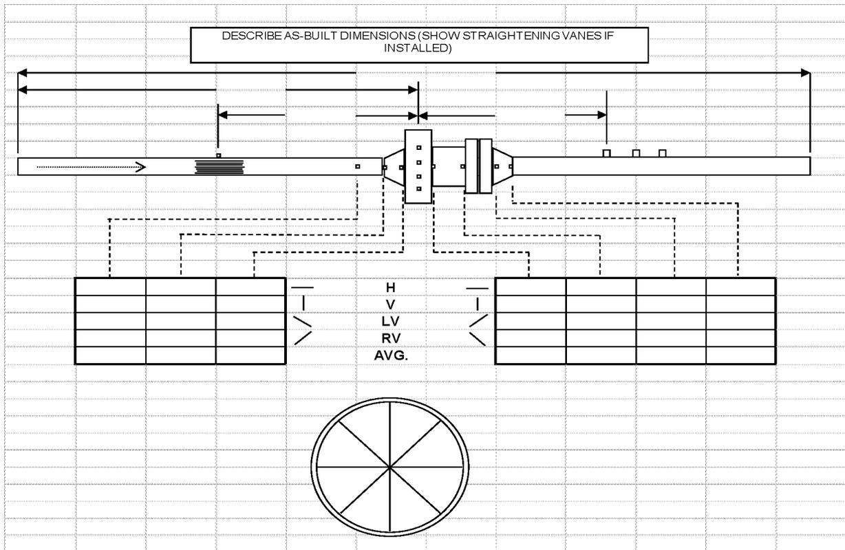
Appendix 1.B– Sample Meter Tube Inspection Form; Simplex Fitting, no Vanes
