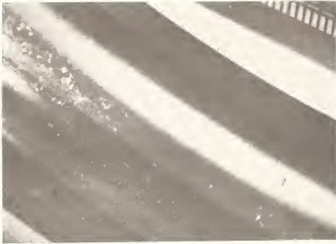
false brinelling on outer race of mast bearing
