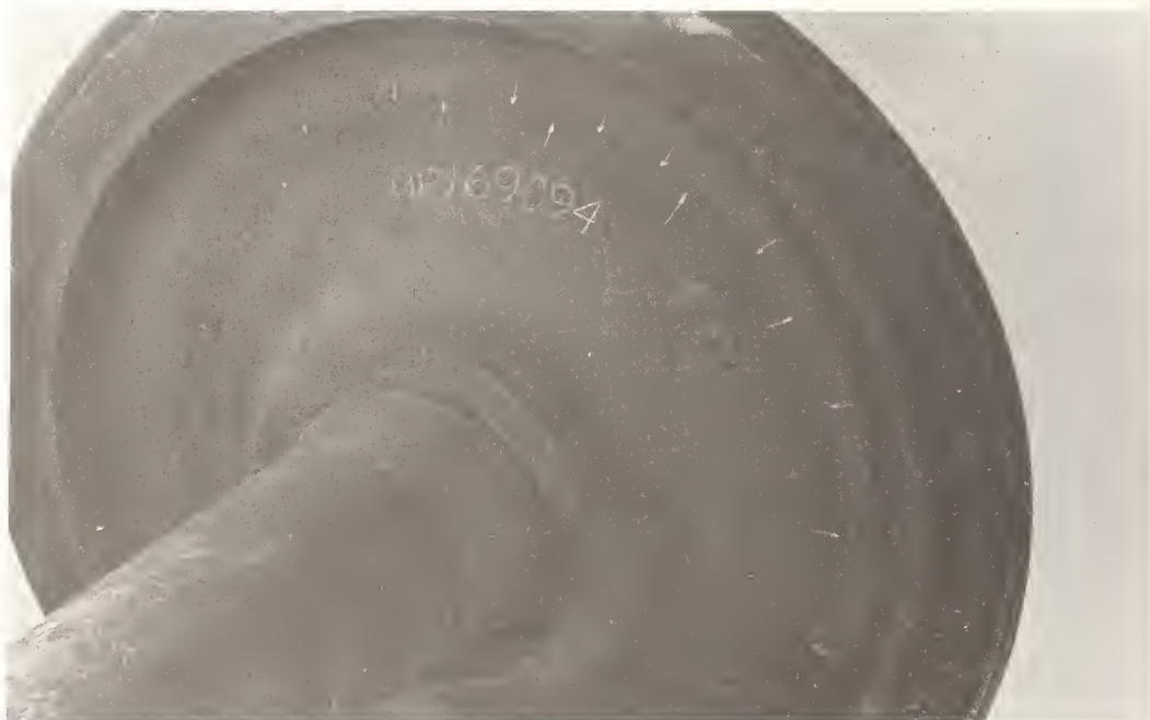
FIGURE 8 PLATE CRACKING FOUND IN THE BACK RIM-PLATE FILLET
