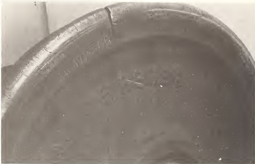
FIGURE 7 WHEEL WITH THERMAL CRACK ON BACK RIM FACE INDUCED BY RETARDER ACTION
