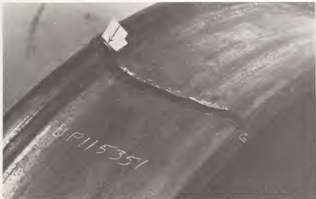
FIGURE 6 THERMAL CRACK DEVELOPED ON THE FLANGE FROM BRAKE SHOE CONTACT
