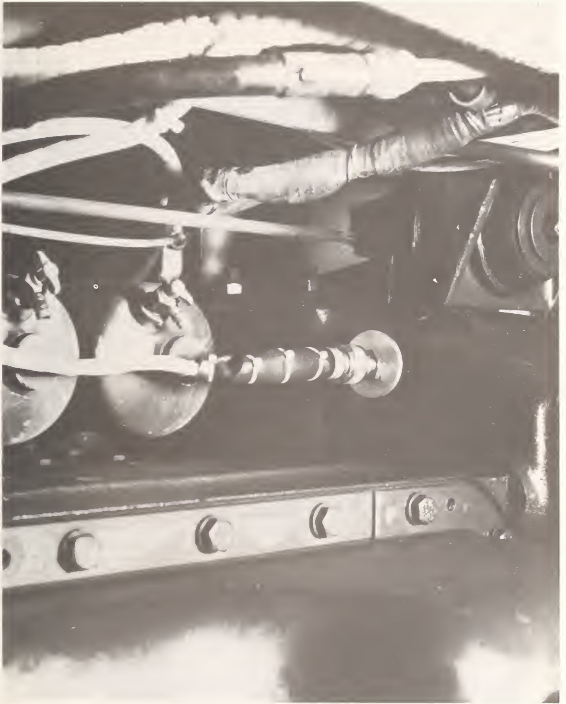
FIGURE 6 ENGINE FLYWHEEL SPEED TRANSDUCER
