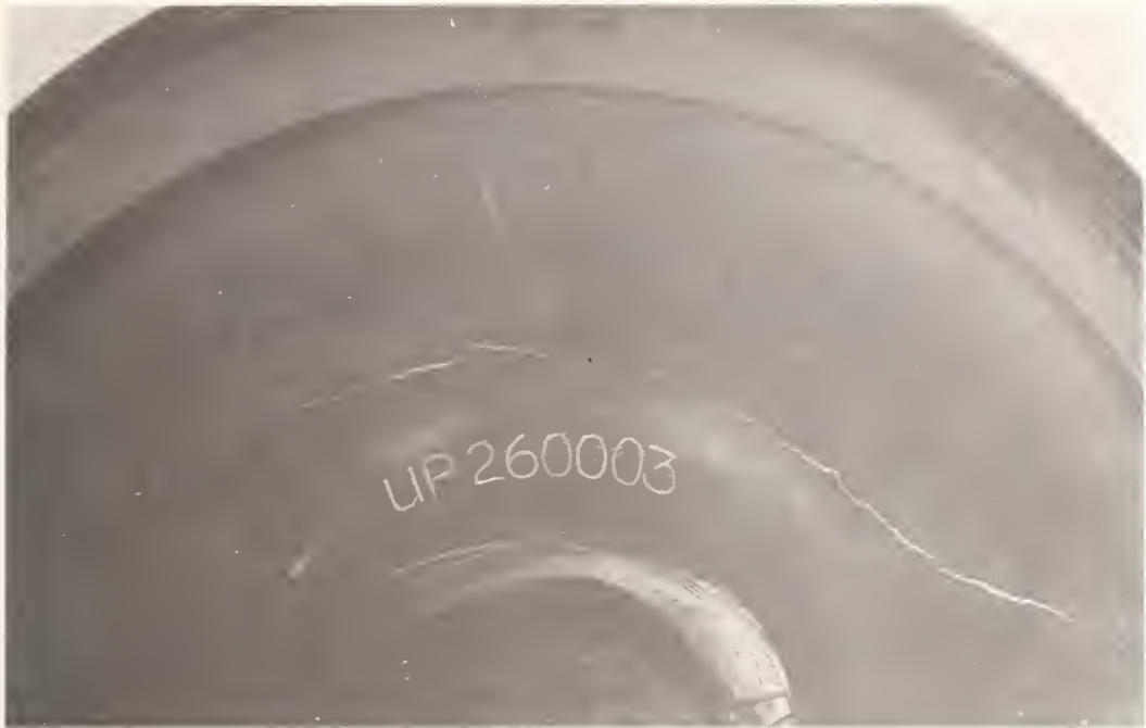
FIGURE 9 PLATE CRACK THAT DEVELOPED IN THE FRONT HUB-PLATE FILLET
