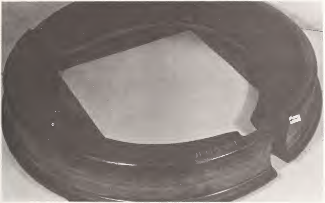
FIGURE 5 WHEEL SHOWING EXTENSIVE BRITTLE FRACTURE INITIATED AT THERMAL CRACK
