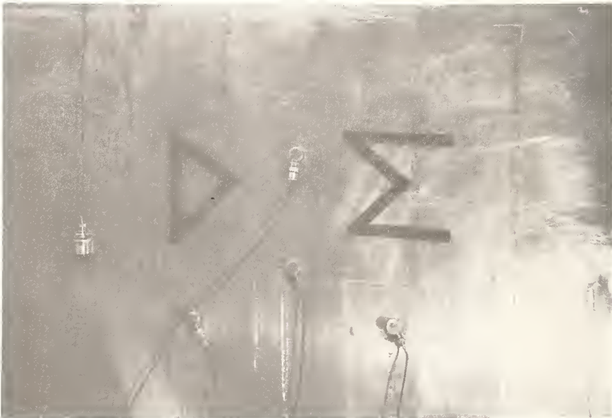
Fig. 6 - Transducer placement on a metal plate and symbols used for illustrating flaw location by acoustic emission multiple channel system
