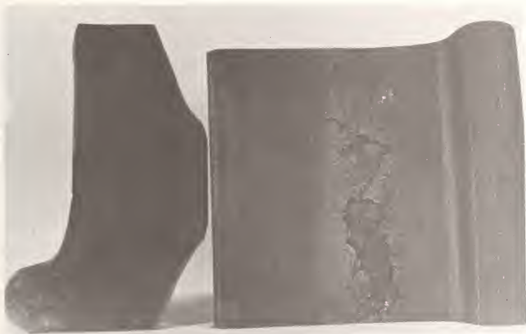
FIGURE 2 PORTION OF A SHELLED WHEEL AFTER DEEP ACID ETCH
