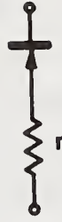
Figure 9. Schematic diagram of the equivalent circuit of a crystal rectifier; case of uniform contact potential.
