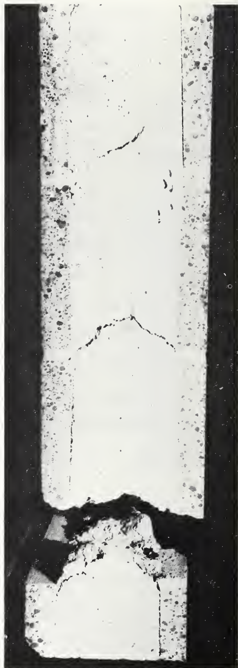
Fig. 20 Grout Bridges and Resulting Failure.
