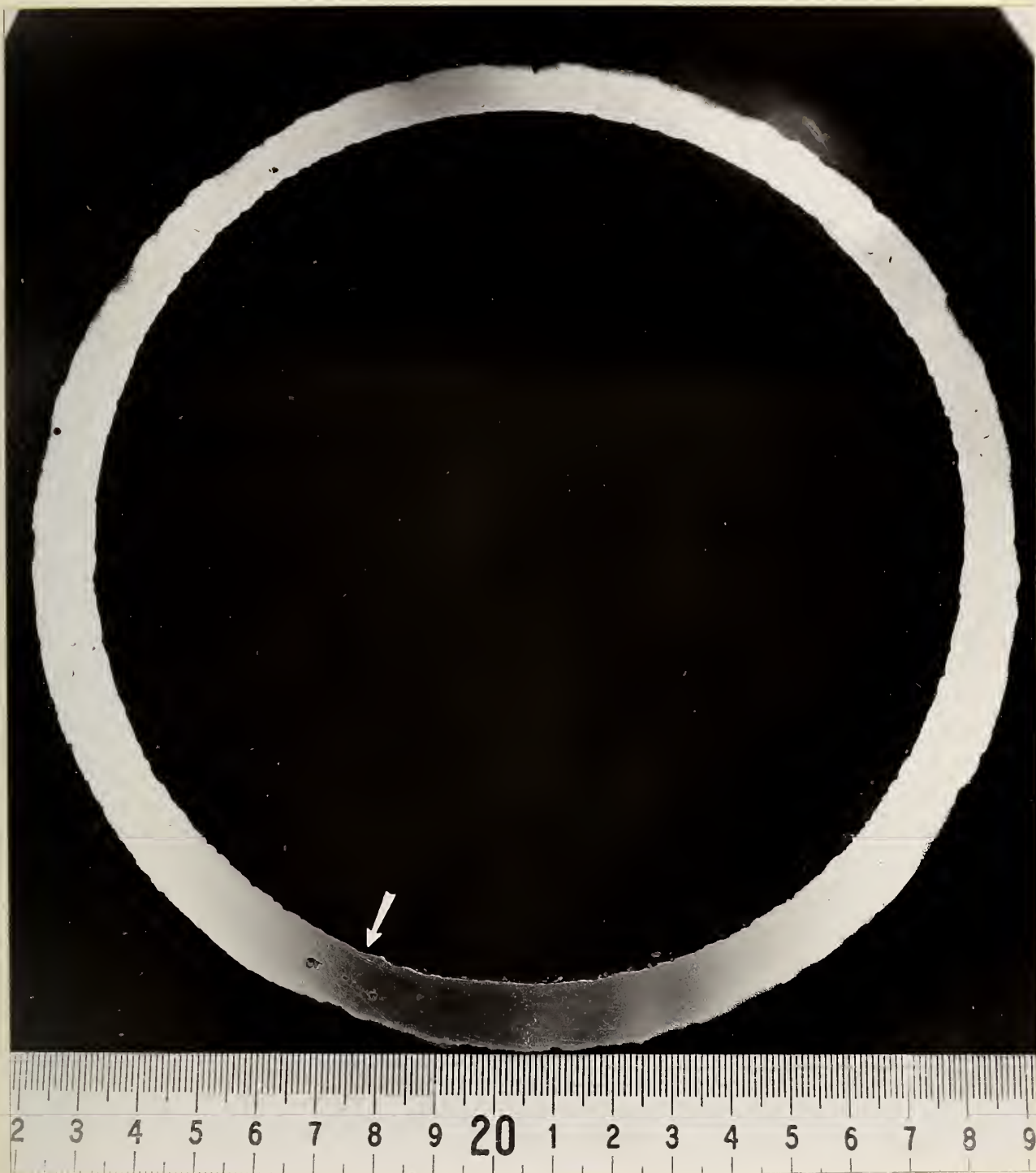
Figure 4. Transverse section through the piece of pipe designated W one inch from the fracture. The top of the pipe is at the top of the photograph. (The notch appearing at the top was put in with a file in order to identify the orientation.) The arrow indicates a region of porosity. X 1
