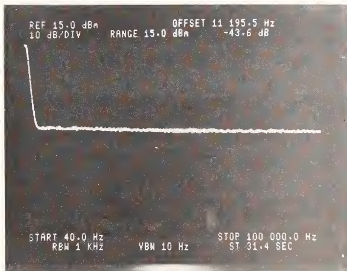
FIGURE 6 - Spectrum Analysis of Received Baseband Signal Using Input of Figure 5
