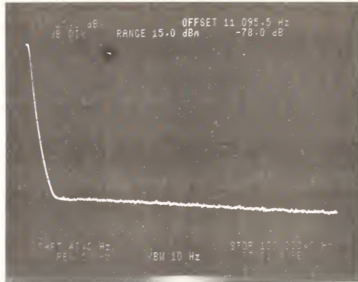
FIGURE 7 - Spectrum Analysis of transmitted baseband signal under operating conditions
