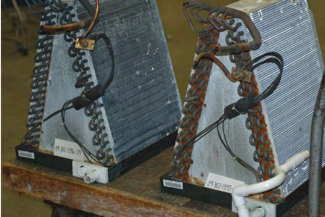
Figure 3 – Photograph of the two air conditioner evaporator coils showing the black discoloration of the copper U-bends and corrosion of the end plate.
