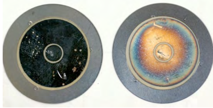
Figure 29 – Comparison of the piezoelectric alarm tone-producing disks from a smoke detector after exposure to the accelerated corrosion-testing environment at Sandia National Laboratory (on left) to one from a detector not exposed to this environment (on right). These photographs were taken after smoke response testing where the one on the left failed to produce a normal tone while the one on the right functioned normally.
