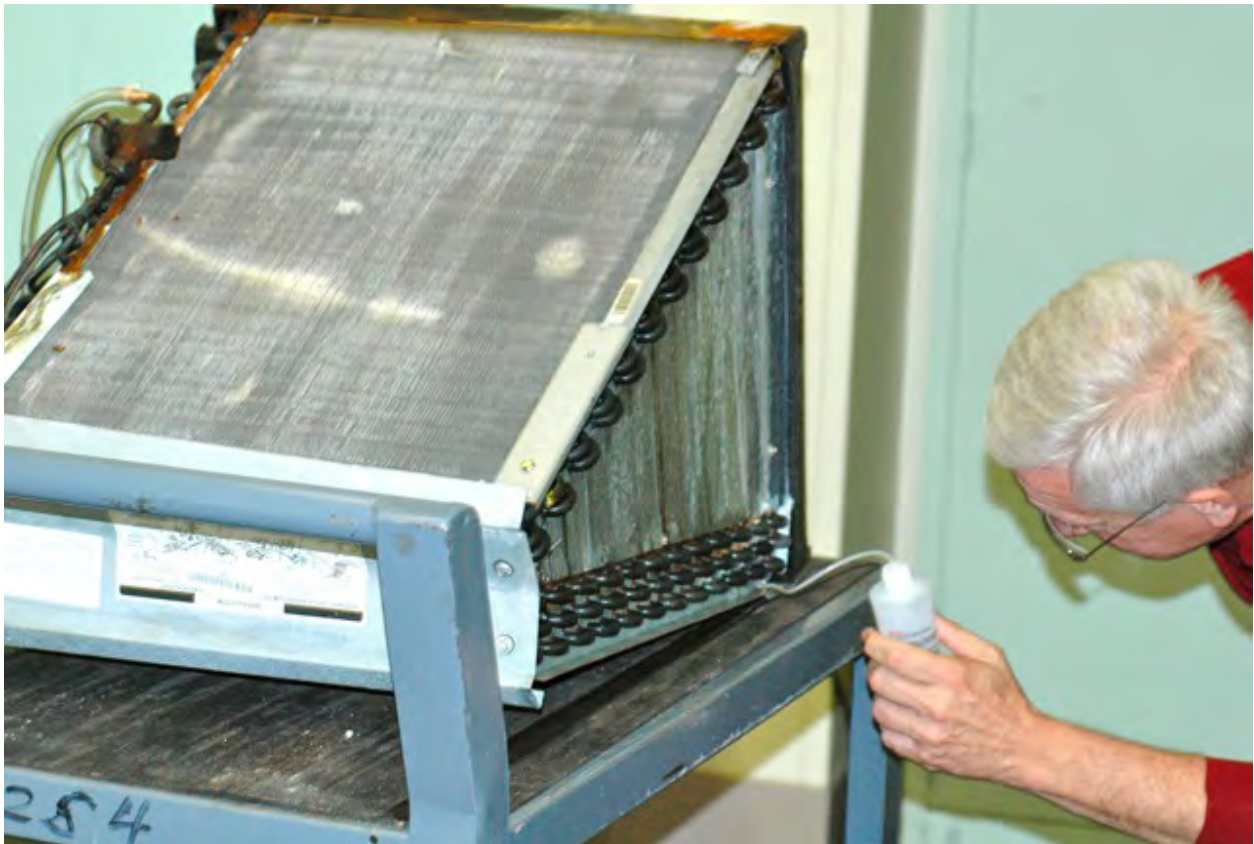
Figure 15 – The garage HVAC unit shown in Figure 13 undergoing leak testing in the metallurgy laboratory at NIST.
