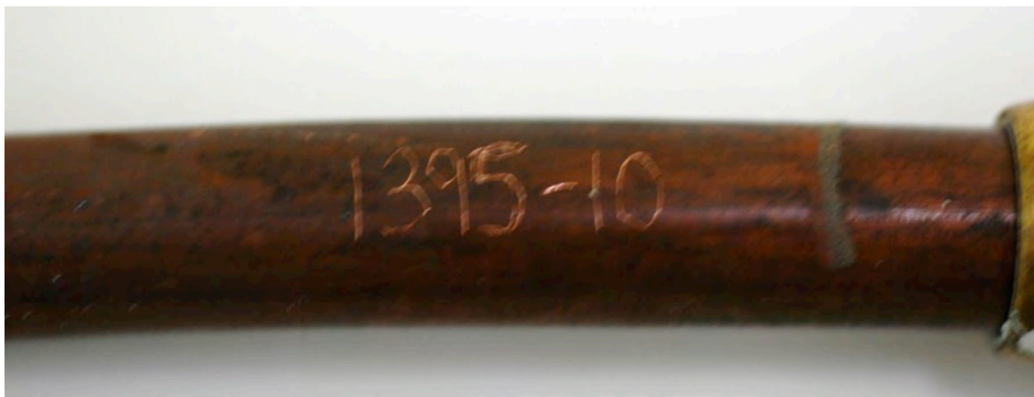
Figure 2 – Scribe marks illustrating the contrast between the color of bare copper and a sample of copper natural gas line tubing.
