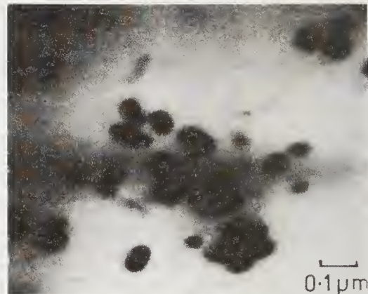
Figure 4. Electron Photomicrograph of Particles in Used Automotive Oil Extract at 100,000 X Magnification. (Note Apparent Agglomeration of Particles.)
