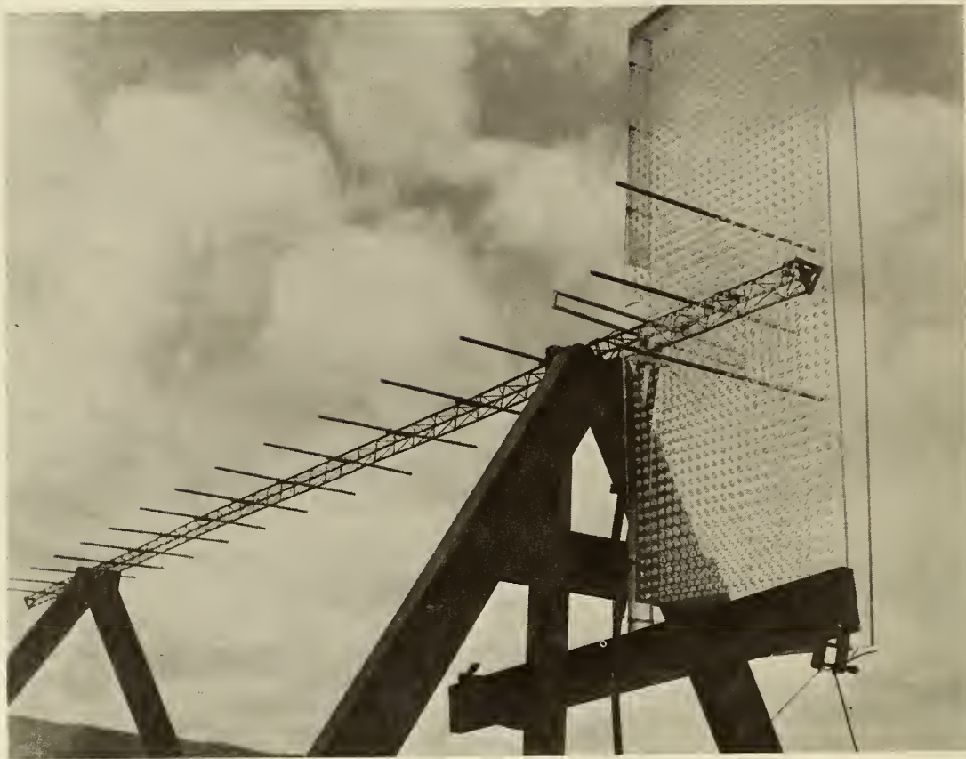
FIG. 3 PHOTOGRAPH OF THE TRIGONAL REFLECTOR EXPERIMENTAL SET-UP USED WITH THE 4.2\lambda YAGI
