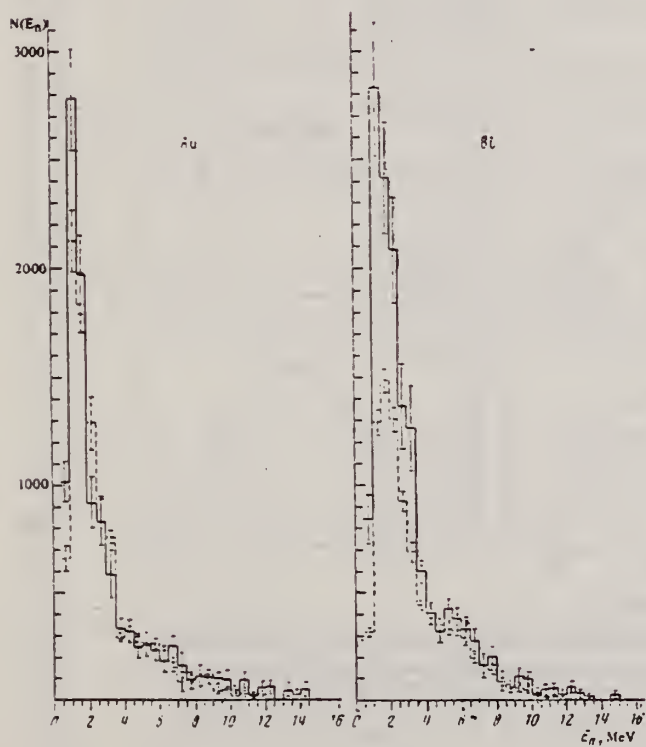
FIG. 3. Photoneutron energy spectra from Rh, Ta, Au, and Bi for irradiation of the samples by bremsstrahlung with maximum energy E_{\gamma \text{ max}} = 20 (dashed line) and 28.5 (solid line) MeV for angles \vartheta with maximum neutron yield. For each nucleus the histograms given for E_{\gamma \text{ max}} = 20 and 28.5 MeV have been combined in the interval E_n = 4-5 MeV.
