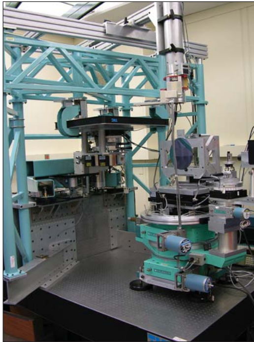
Figure 2. Ceramics Division Parallel Beam Diffractometer (CDPBD). Showing rotating anode source (center left), monochromator / optics platform (upper center), diffraction goniometer (lower right), receiving optics/detector (center right), and cable managing goniometer (top center).
