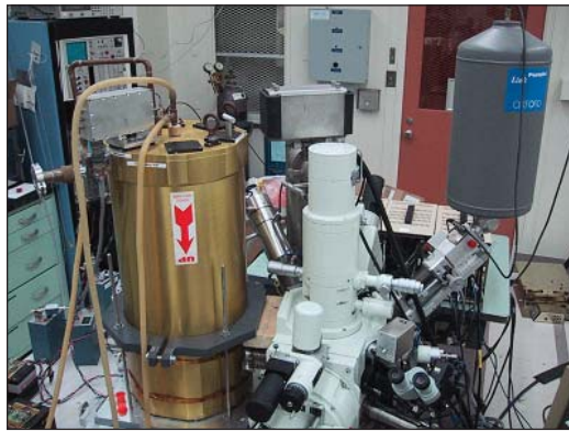
Figure 1. Single-pixel NIST X-ray microcalorimeter system on a scanning-electron microscope. The system was developed in the Electronics and Electrical Engineering Laboratory (EEEL) at NIST, Boulder, and transferred to the Chemical Science and Technology Laboratory (CSTL) at NIST Gaithersburg to be used to study problems of interest to the semiconductor industry.
