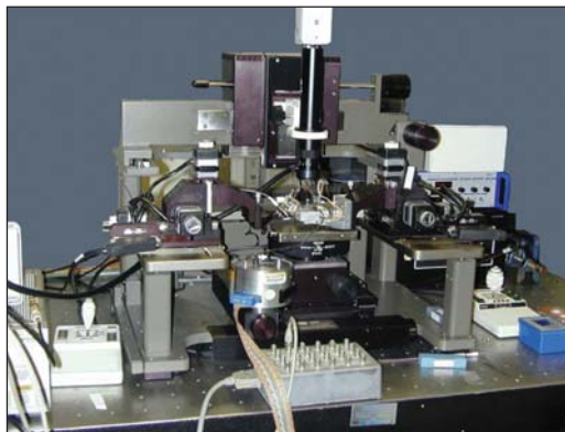
Figure 1. Universal test bed for electric and magnetic field probing on a nanoscale.
