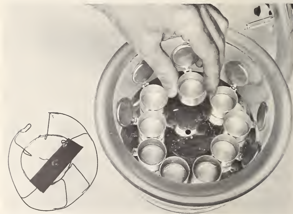
Isopiestic vapor pressure measurements provide a new technique for measuring the thermodynamic properties of aqueous solutions containing one electrolyte and one non-electrolyte. The wire apparatus is used to close the covers on the sample cups while they are still under vacuum in the dessicator. (See p. 91.)
