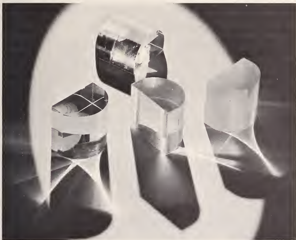
A new method of producing glass with controlled light scattering properties led to these prototype turbidity standards. They are now being studied as possible replacements for the less durable plastic and liquid standards presently in use. (See p. 11.)
