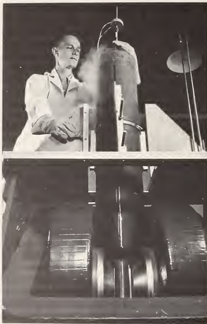
Cryostat and magnet used in investigating superconductivity in thin films. (See p. 180.)
