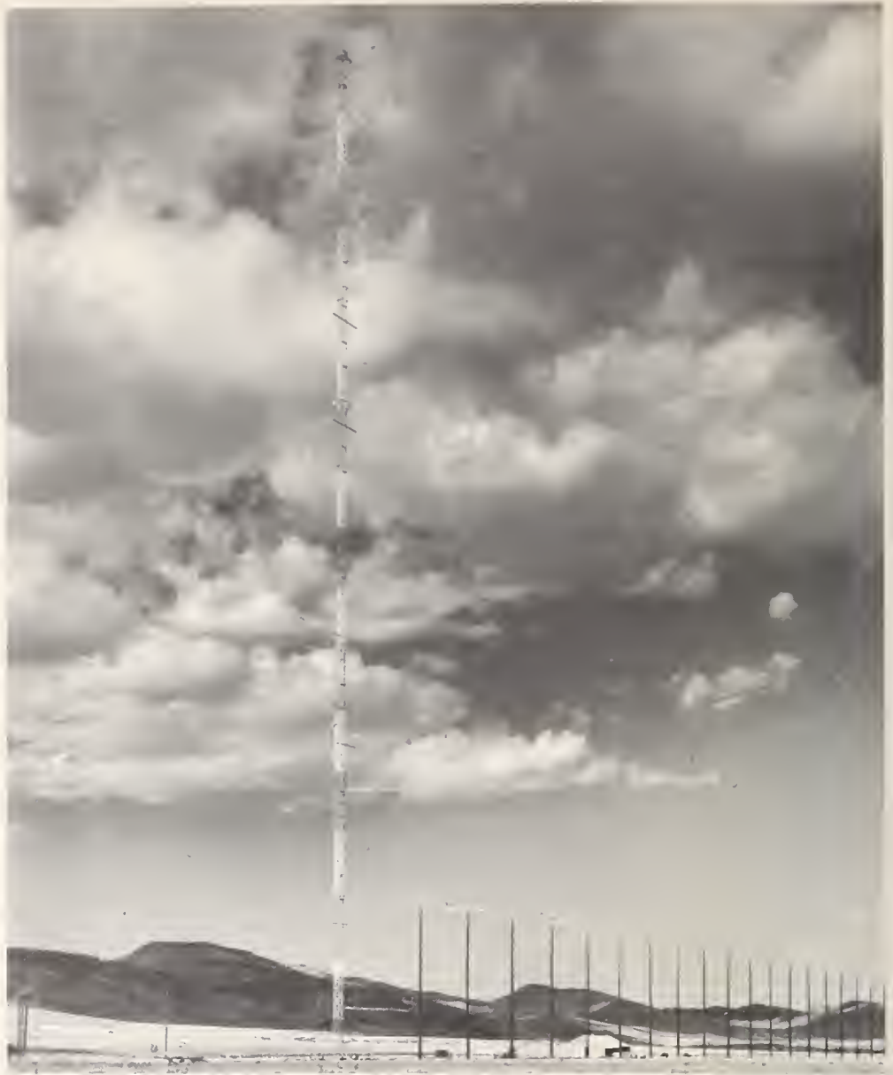
Azimuthal and elevation electronically-scanned arrays at the NBS Table Mesa (Colo.) field site are used in high-frequency ionospheric propagation studies. (See p. 163.)
