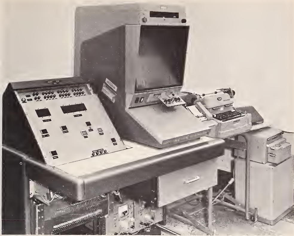
Information handling system designed for the Naval Intelligence Agency as a low-cost means of storing, searching, and retrieving intelligence data. (See p. 136.)
