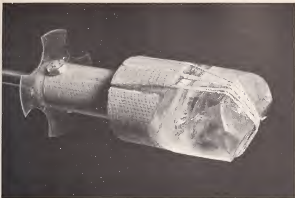
Holmium ethyl sulfate crystal used to measure the dependence of the yield of photoneutrons from holmium on the orientation of the nucleus with respect to the photon beam direction. Nuclei were aligned by cooling the crystal to 0.29^\circ \text{K} . (See p. 82.)
