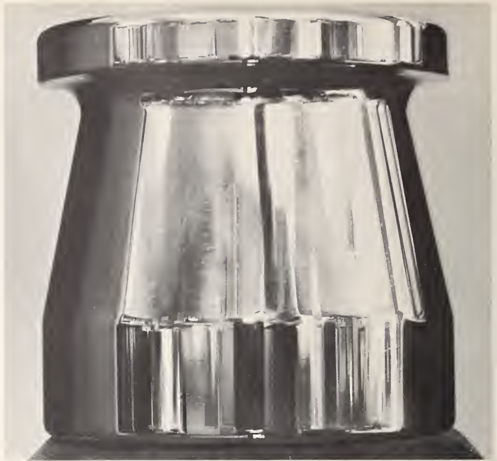
New design for mass standards made of stainless steel. A metric set of this design is being acquired for the Latin American standards program. (See p. 195.)
