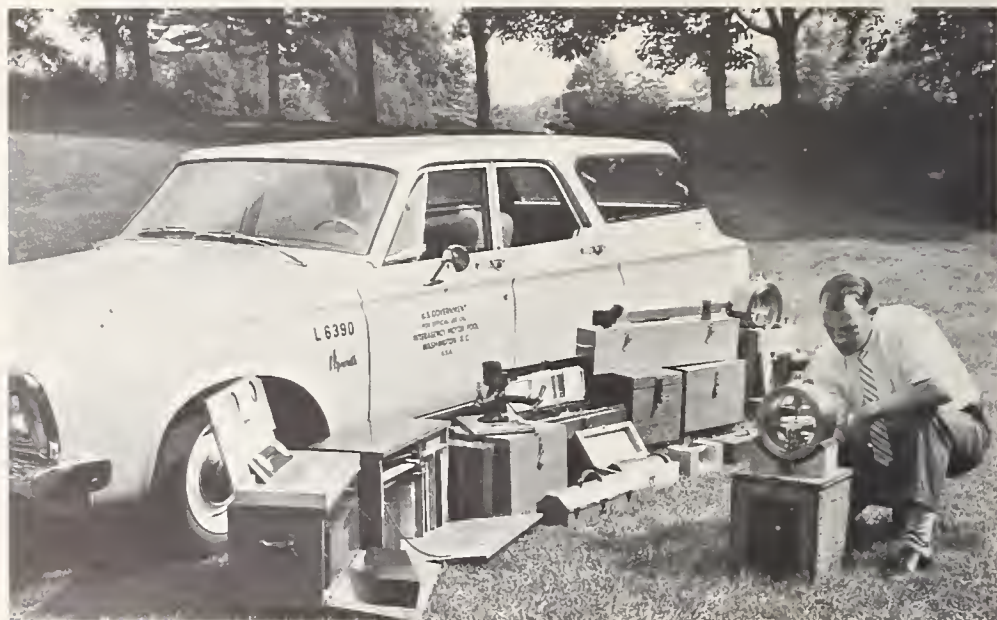
One of three sets of equipment used to check cement and concrete testing apparatus by the NBS Cement and Concrete Reference Laboratory in a joint U.S. Government—ASTM program. The service is available throughout the United States and Canada.
