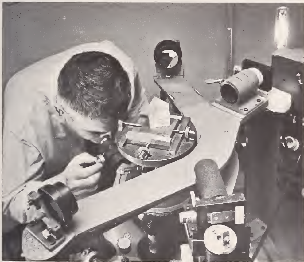
Measuring the refractive indices of synthetic calcium fluoride. Such values provide a basis for selecting optimum crystalline materials for the design of optical components and systems. (See p. 30.)
