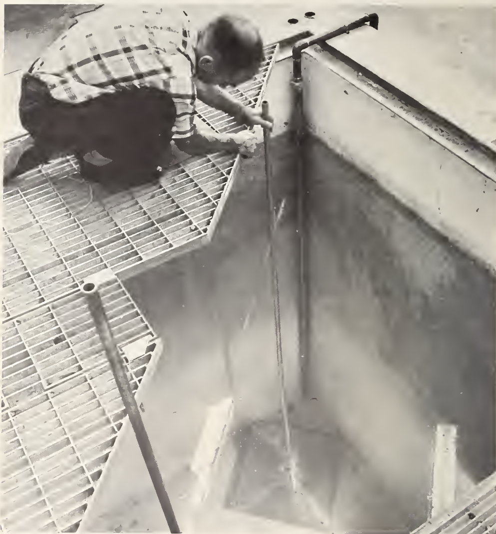
Placing a monomer sample into a cobalt 60 radiation source 10 feet under water ( lower center ). Under the influence of the gamma radiation, high pressures, and high temperatures, several monomers which do not ordinarily form polymers have been polymerized. Polymers of unusual or novel structure with unique properties may be produced by such studies. (See p. 122.)
