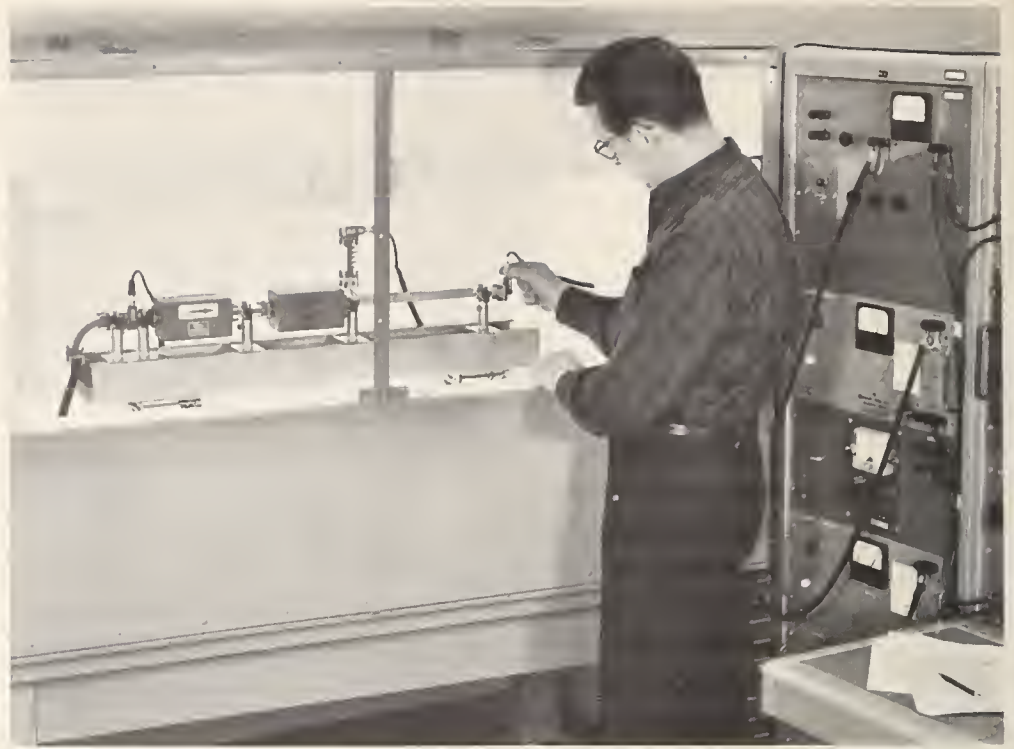
A new transfer instrument, designed and built by the Bureau, is used for the intercomparison of microwave power meters. A bolometer unit is being calibrated. The insulated chamber (which is normally closed) stabilizes the temperature around the equipment. (See p. 64.)
