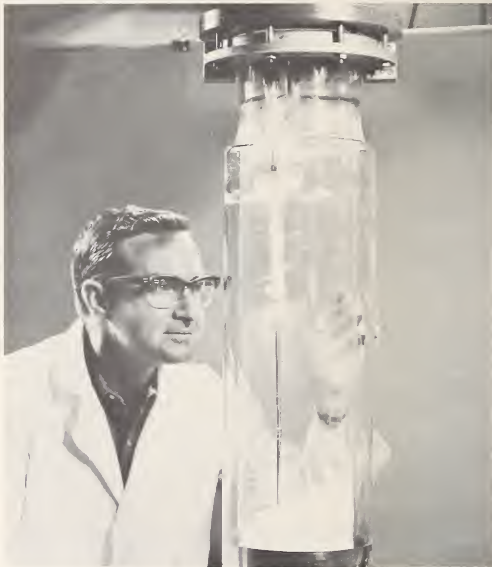
Investigation of cryopropellant freezing phenomena. Propellants leaking or venting in low-pressure environments may cause solids to form in critical regions, resulting in possible failure of space vehicle propellant systems. (See p. 184.)
