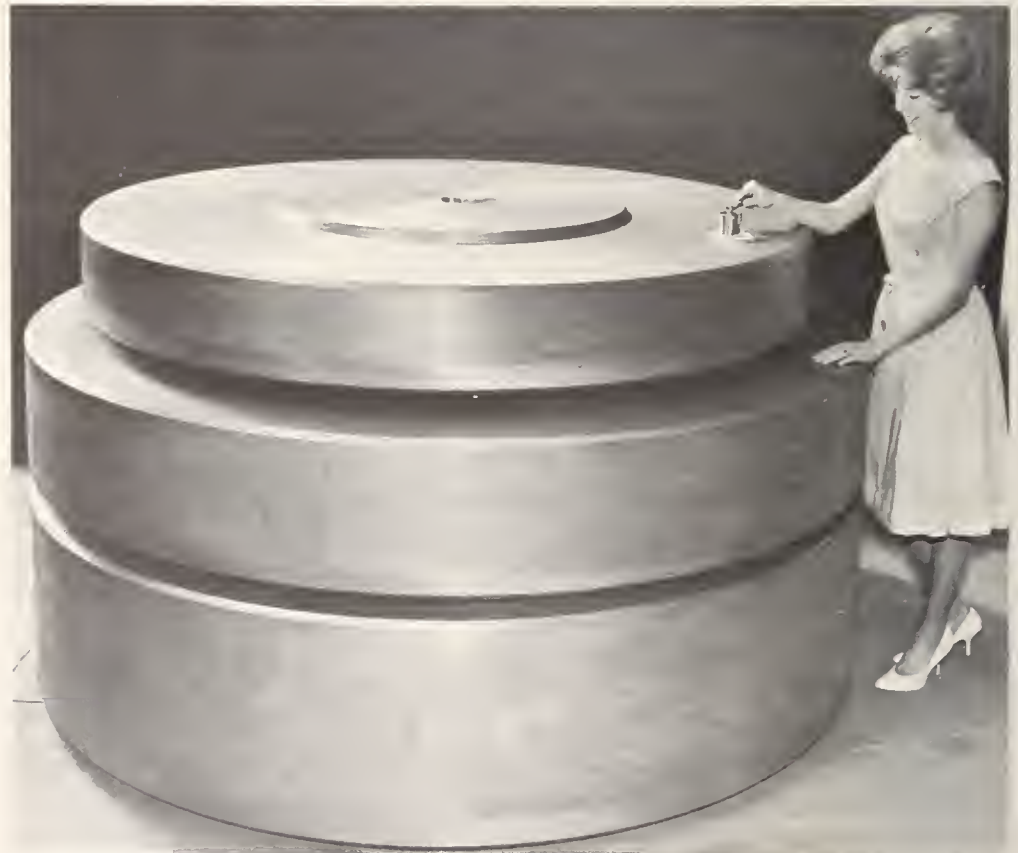
Ten-, twenty-, and thirty-thousand pound mass standards compared to a one-kilogram mass. These weights, the largest ever constructed to meet NBS Class C requirements, will be used in the deadweight force machines now under construction at the new Gaithersburg laboratories. (See p. 40.)
