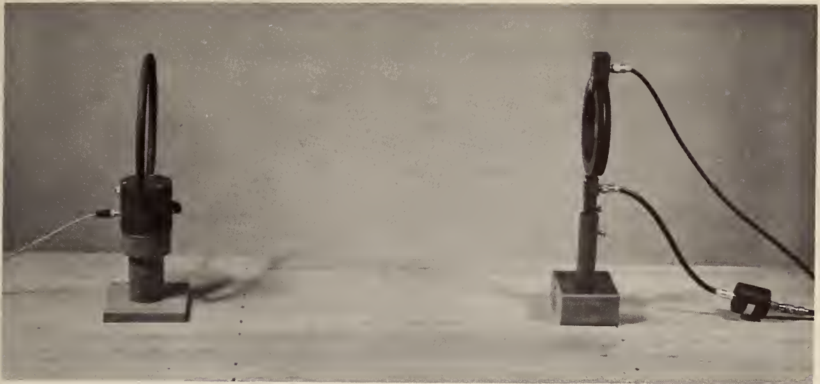
Figure 5.11. Loops Positioned for Calibration.
