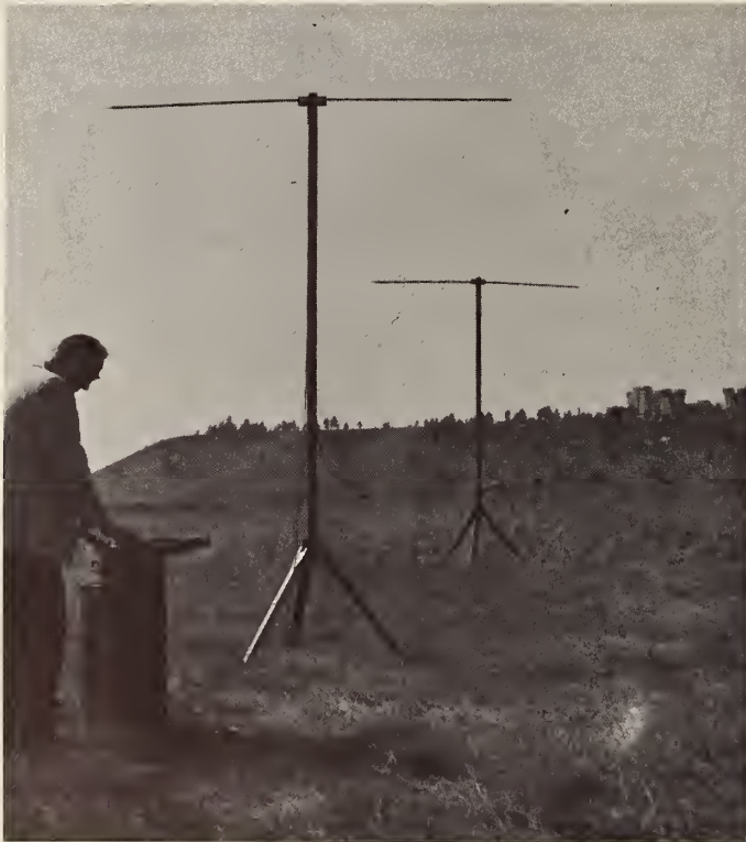
Figure 6.12. Typical Field Calibration Setup for Dipole Antennas.
