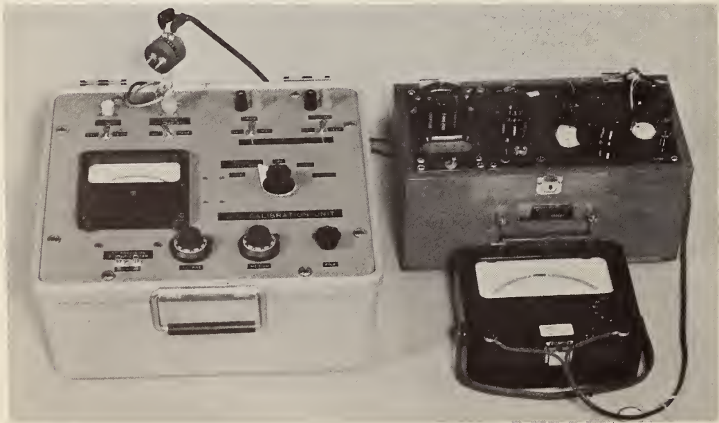
Figure 6.13(a). Diagram Showing the DC Calibration of the Dipole Voltage Standard.
