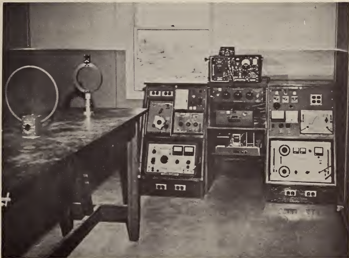
Figure 5.5. Typical Loop Calibration Setup at NBS.
