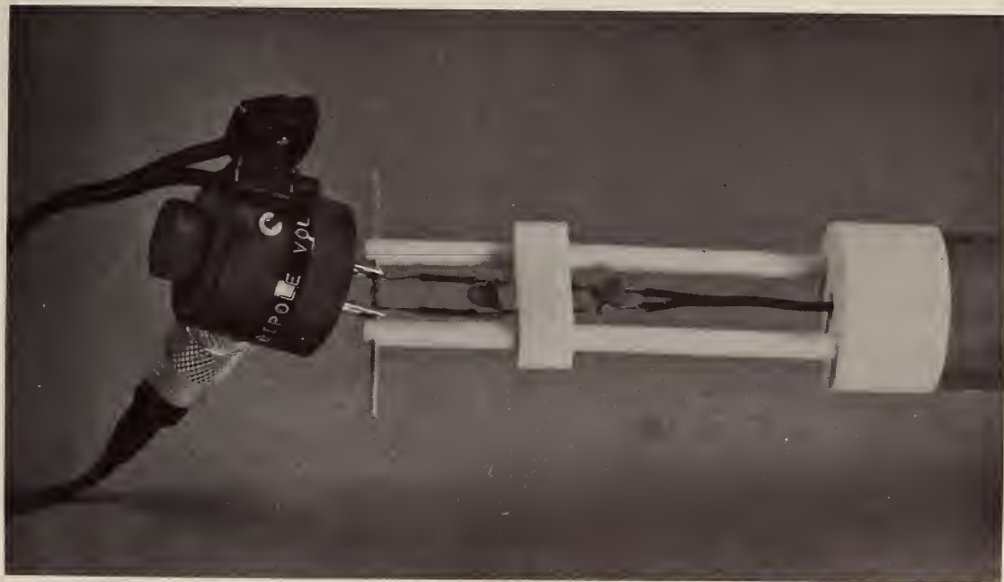
Figure 6.7. Balanced Voltage Standard Attached to Crystal Diode Mounted in Antenna.
