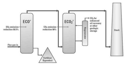
Incorporation of Powerspan's ECO $_2$ ® carbon capture process with the commercially available multi-pollutant control ECO $_2$ ® process.
